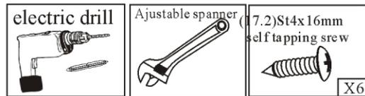
Carry backboard and glass room on the tub, adjust place, then use 3 mm drill to dig holes, tighten with (17.2) self tapping srew.
