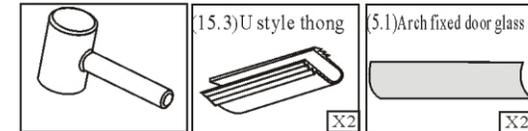
Insert U style thong to arch fixed door glass, put on the rails and knock it to socket of side upright column with rubber hammer.
