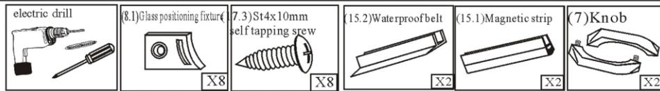
Put knob into movable door's hole, tighten with screws. Fix glass positioning fixture with self tapping screw, then insert waterproof belt and magnetic belt.
