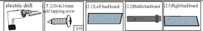
To align three pieces of backboard, dig holes with 3mm drill bit, tighten with (17.2) Self tapping screws. hypodispersion
